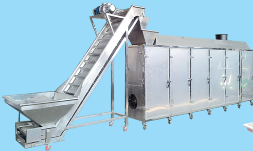
Natural wind multi-layer air drying assembly line
